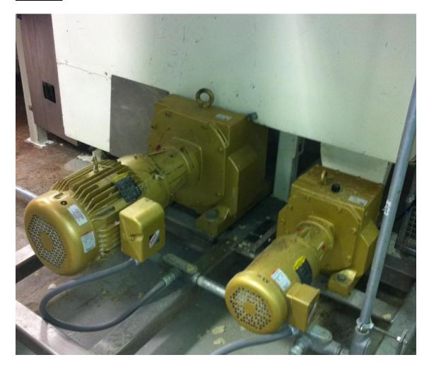
The customer purchased a package through Baldor's System-1 group that provided a tighter speed range and allowed them to minimize upgrading to a larger HP solution. The solution is more energy efficient, more cost effective, and as an added bonus, the customer can separately control the conveyor belt speed and the extruder roll speed.
