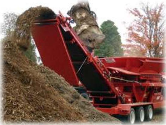
Mechanically powered wood hogs can be portable, being mounted on wheels on frames suitable for towing behind a truck or van. For mobile hogs, power is generally provided by an internal combustion diesel engine from 5 to 1,200 horsepower.
