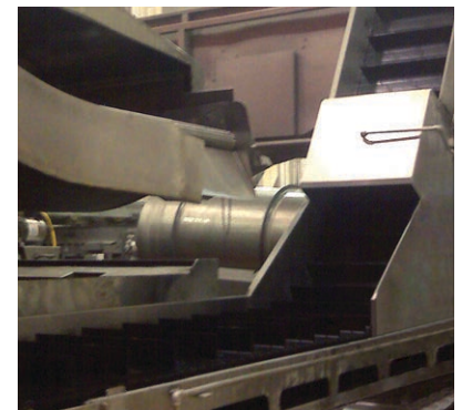
The Rexnord MatTop FTR R8506 Chain handles temperatures up to 325 F.
